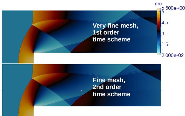
Figure 10. Comparison of flow patterns (density) for the case calculated with the first order of approximation with respect to time on the finest mesh, and for the case calculated with the second order of approximation
