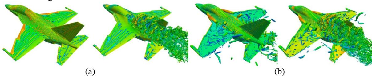
**Figure 9.** Instantaneous vortex structures (iso-surface of  $Q$ -criterion) of flow around an aircraft with and without airbrake at angles of attack: (a)  $\alpha = 0^\circ$ ; (b)  $\alpha = 20^\circ$
