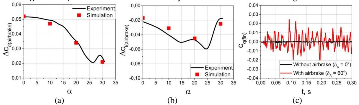
**Figure 8.** The influence of the airbrake release on the change of aerodynamic coefficients: (a) drag; (b) lift; (c) lateral force on the tail fin ( $\alpha=0^\circ$ )
