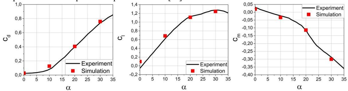
**Figure 7.** Dependence of the aircraft's aerodynamics characteristics on the angle of attack
